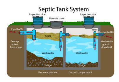
The accumulated solids in the bottom of the septic tank should be pumped out **every 3 to 5 years.** This prolongs the life of your system. Septic systems must be maintained in order to work properly and to keep them from failing. Septic tanks equipped with effluent **filters should be cleaned once a year. Resting lines or bull run valves should also be charged** at this time.
