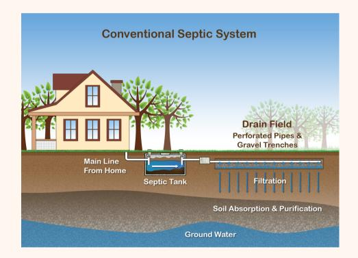
A **septic system** consists of a **septic tank**, **distribution boxes** and a **drain field**, all connected by pipes called **conveyance lines**.
